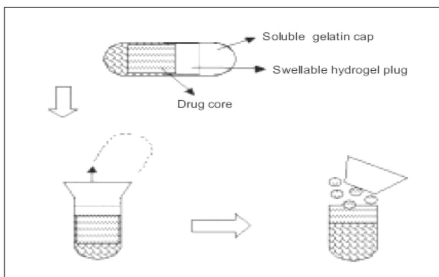
**Fig. 2: Design of Pulsincap system.**
