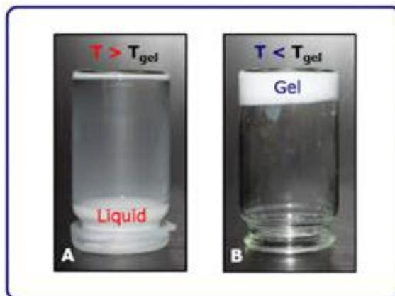
Fig. 3 Temperature induced In-Situ gelling system.<sup>[4]</sup>
