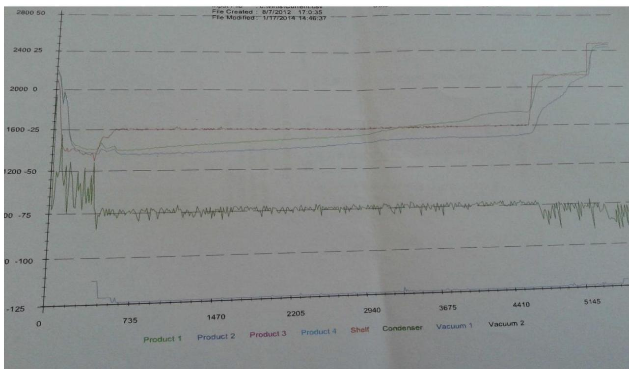
Graph of lyophilization cycle representing the drying of solution on different temperature and chamber pressure with respect to time.
