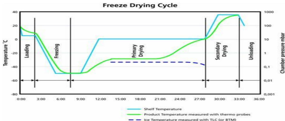
**Fig :** A typical freeze drying cycle showing shelf temperature, product temperature on different time under pressure in mbar.
