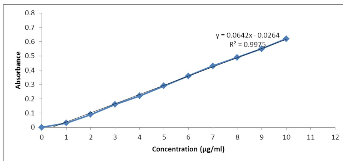
Fig. 1: Standard Calibration Curve of Candesartan cilexetil.
