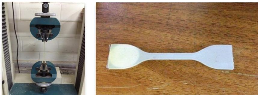
**Fig.1: Sample Cut into Dumbbell Shape for Mechanical Properties Estimation and Photographs of Texture Analyzer Instrument While Measuring the Mechanical Properties.**
