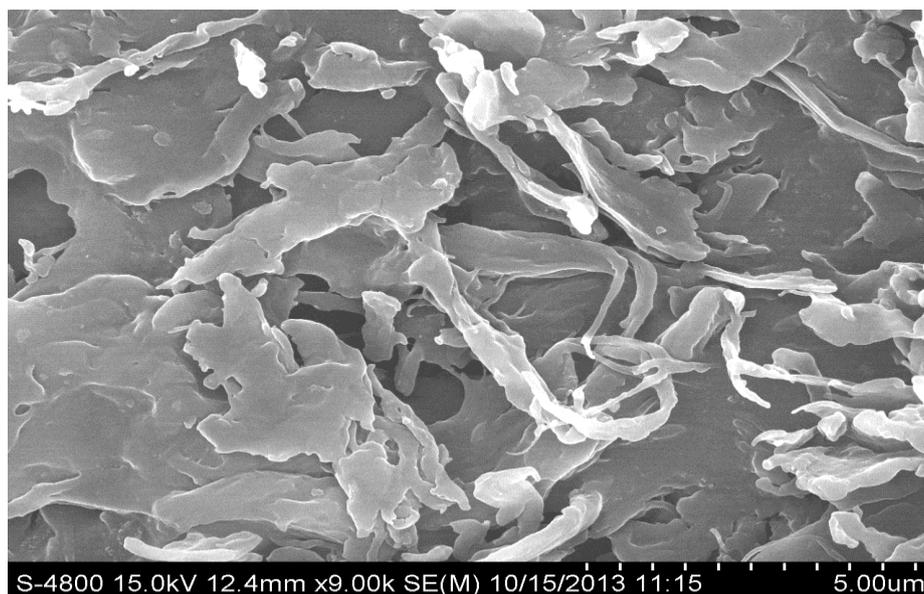
**Fig: 3 SEM image of Chitosan-g-MAN composite**
