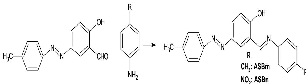
Scheme 2. Preparation of azo Schiff bases.
