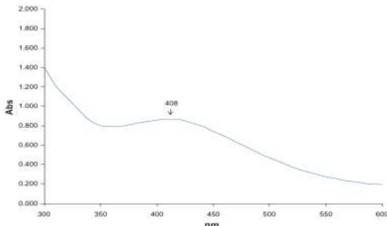
**Figure.2. UV-Visible spectrum of AgNPs**
