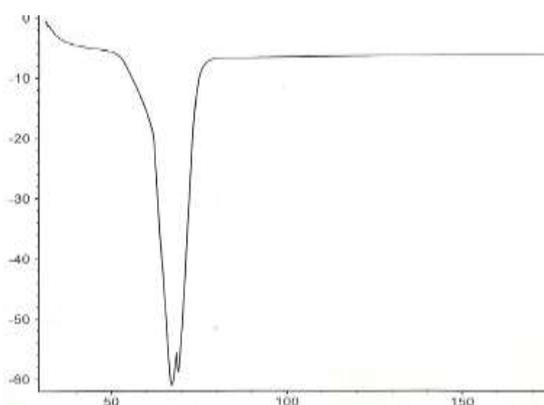
**Fig. 1e. DSC thermogram of PEG alone**
