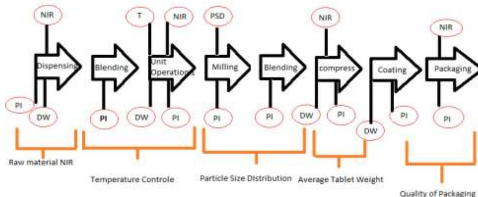
**Figure 1** illustrates a typical tablet manufacturing process in a pharmaceutical process.
