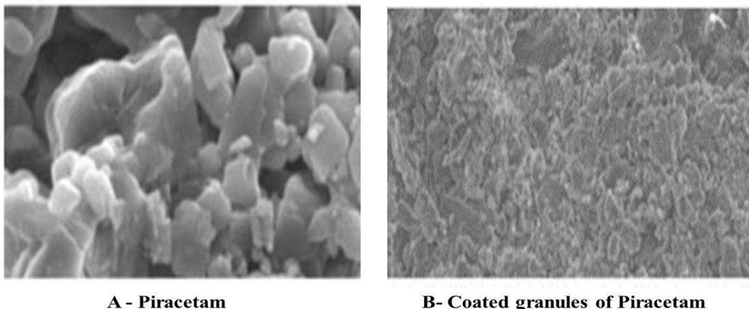
**Fig. 4:** SEM images for A) Piracetam pure drug and B) coated granule of Piracetam.
