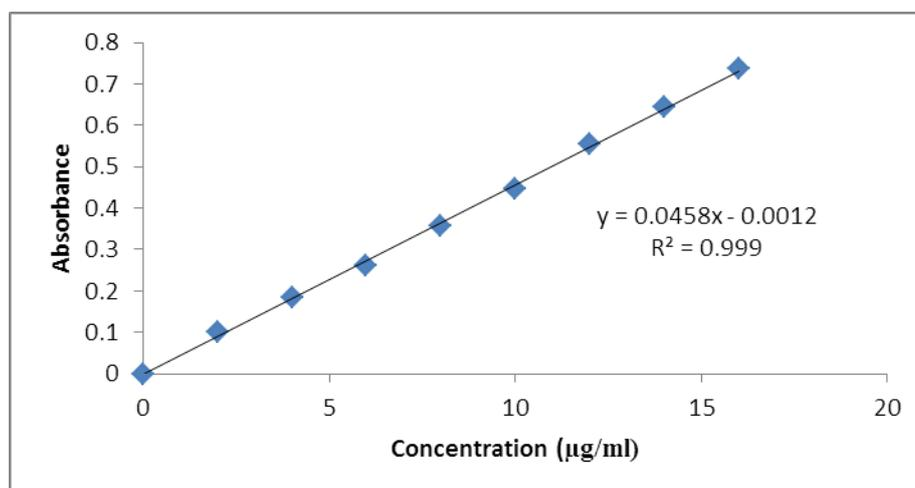
**Figure 4: Standard calibration curve of ondesartan hydrochloride.**
