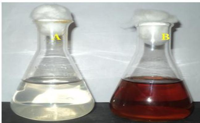
**Fig.1: Aqueous solution of 1mM AgNO<sub>3</sub> (B) Silver nanoparticles.**
