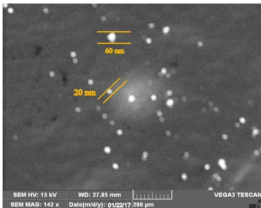
**Fig.4: High resolution scanning electron microscopic (SEM) image of silver nanoparticles (AgNPs). Polydispersed AgNPs ranged between 20–60 nm.**
