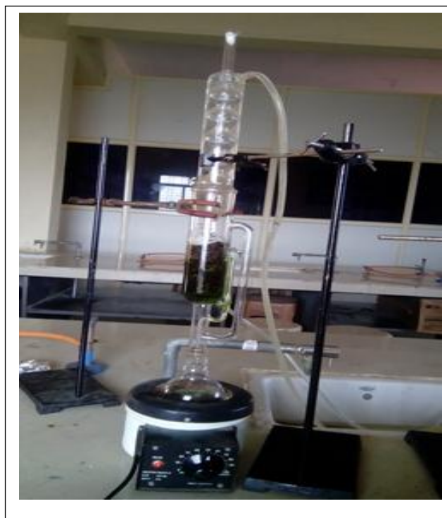
Fig.2: Extraction preparation by soxhlet apparatus.
