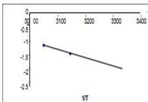
**Figure 8: Plot of log k  $V_s$   $1/T$  to determine k at  $T_{25}^{\circ}\text{C}$ .**
