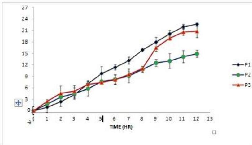
**Figure 6: Cumulative drug release profile of piperine from phytosomal cream formulations (P1, P2, P3) diffused into buffer solution of pH6.6 detected at 344 nm. Results are expressed as mean ± SD when= 6.**
