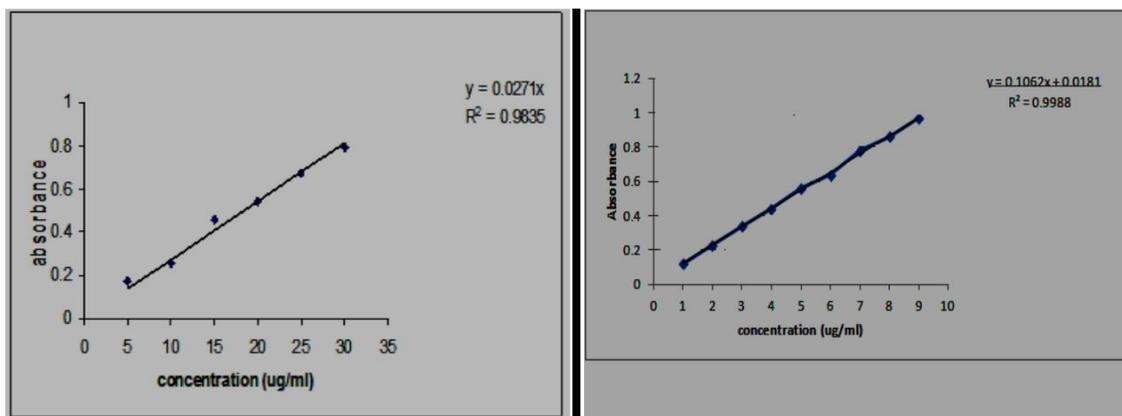
Figure 1: Standard calibration curves for Piperine at  $\lambda_{\text{max}}$  344nm in ethanol, (left) and right (buffer pH 6.6)  $n=6$ .
