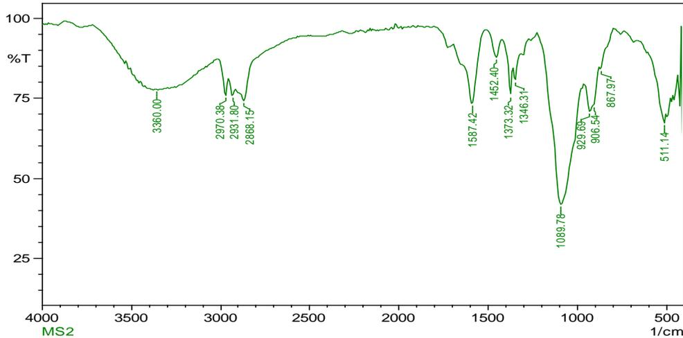
**Figure-1b: FTIR Spectral details of NCS/PU/PPG-glu(1:1:1)ternary blend.**
