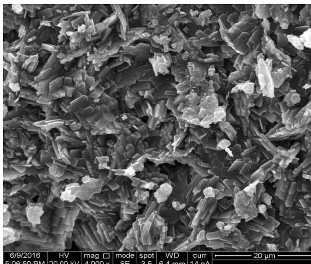
**Figure 4b: SEM Micrograph for NCS/PU/PPG-glu(1:1:1) ternary blends.**
