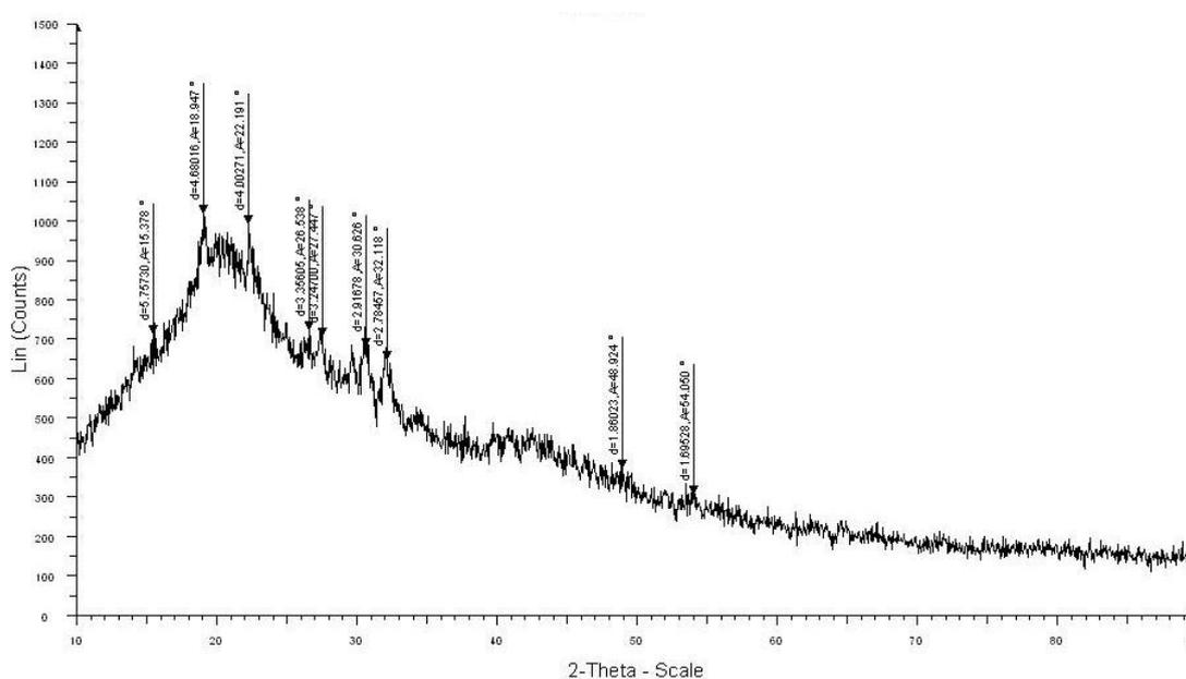
Figure 3b: XRD details of NCS/PU/PPG-glu(1:1:1) ternary blends.
