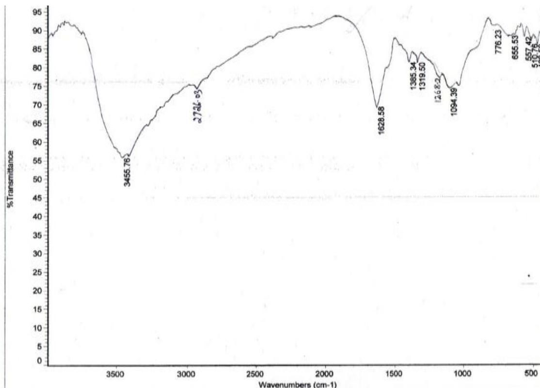
Figure 1a: FTIR Spectral details of nanochitosan (NCS).
