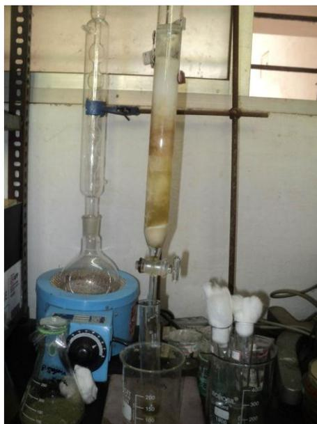
**Fig. 3: Column chromatography Setup.**
