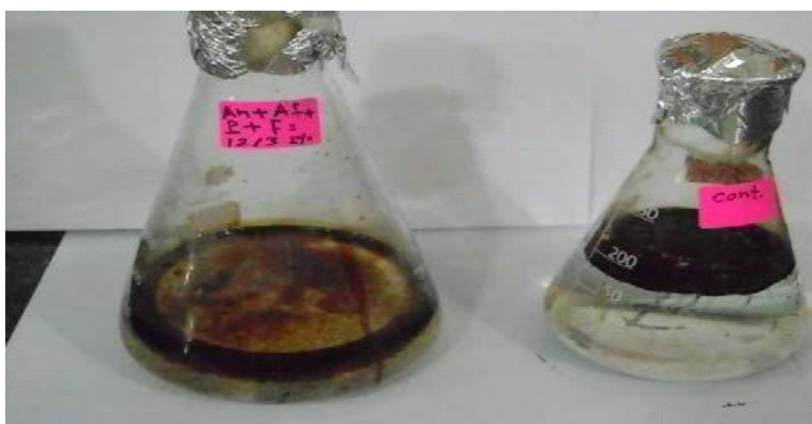
Figure (9): Biodegradation of crude oil by A. niger , A. fumigates , F. avenaceium and P. funiculosum after 28 day incubation.
