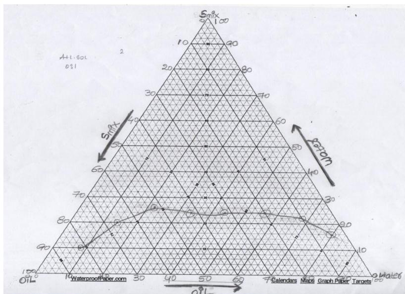
**Fig. 3(c): Ternary phase diagram of 2:1 ratio of Arachis oil : s mix (labrasol:PEG 400) water.**
