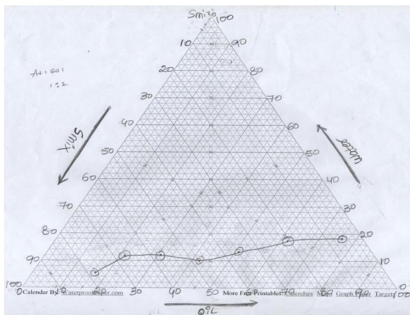
**Fig. 3(b):** Ternary phase diagram of 1:2 ratio of Arachis oil : s mix (labrasol:PEG 400) and water.
