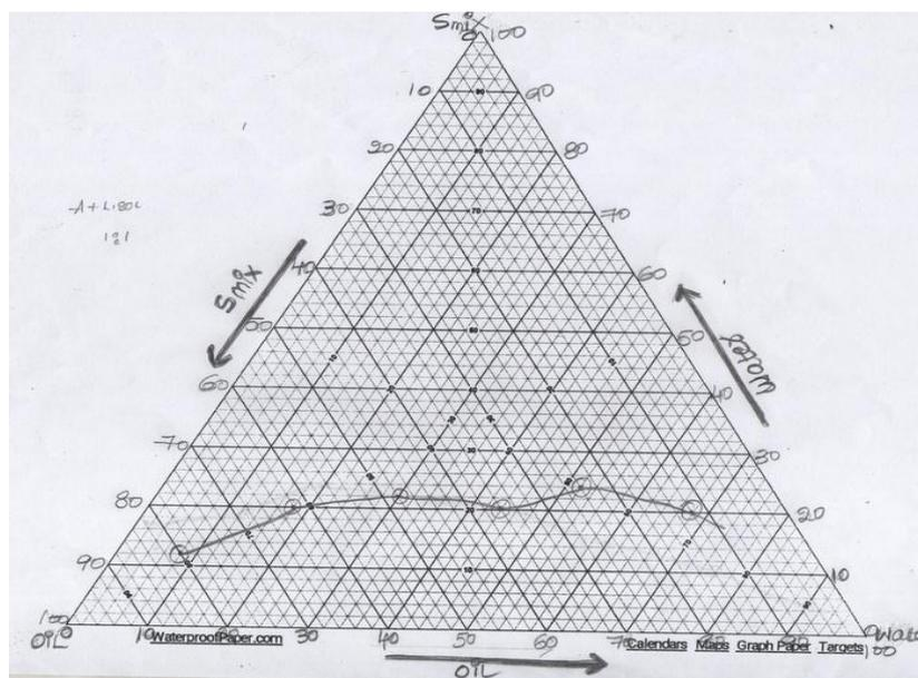
**Fig. 3(a)** Ternary phase diagram of 1:1 ratio of Arachis oil : Smix (labrasol:PEG 400) and water.
