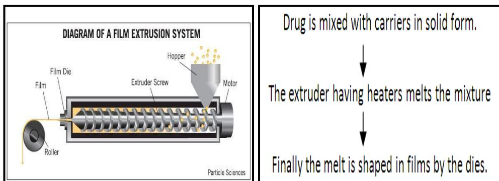
**Fig. 2: Film extrusion apparatus and procedure.**<sup>[5]</sup>
