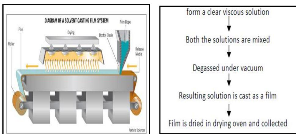
**Fig. 1: Solvent casting apparatus and procedure.**<sup>[5]</sup>
