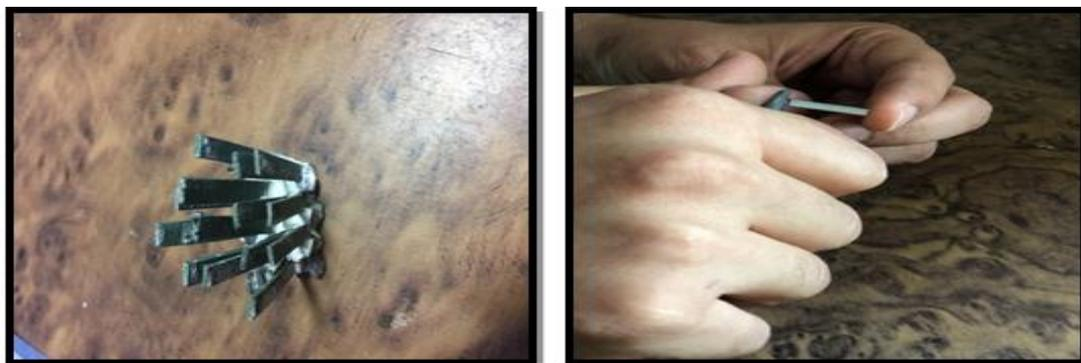
**Figure (5): (a) divesting after casting, (b) smoothing the metal sample.**
