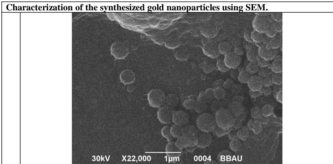
**Figure 4: Characterization of the synthesized gold nanoparticles using SEM.**
