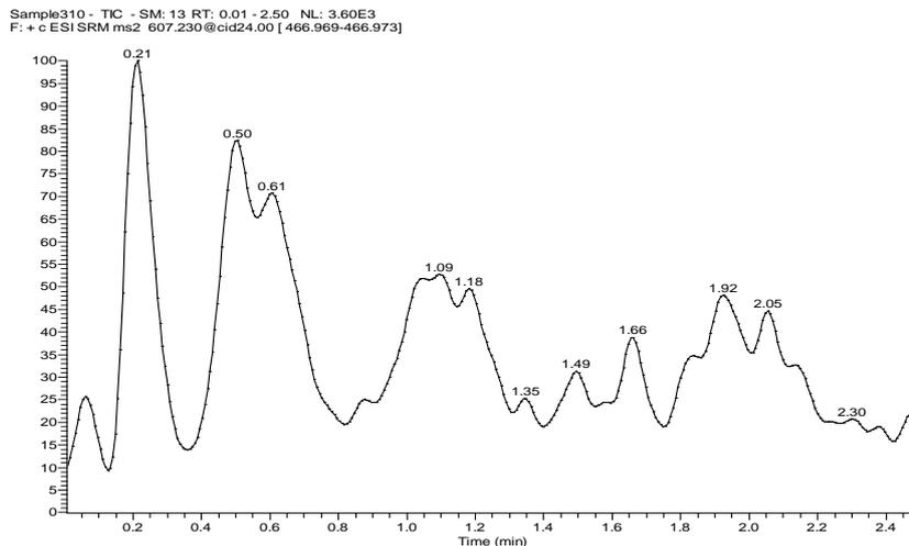
**Figure 3: Representative chromatogram of Clofarabine extracted from Blank plasma sample.**
