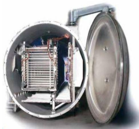
**Fig:5 Freeze Dryer (open)**
