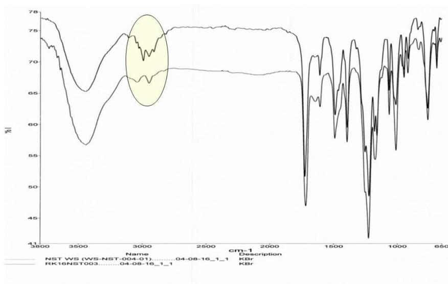
**Figure 4: Sample overlay spectra with Standard – Noise in sample at Circled part.**
