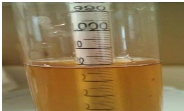
**Fig 27: The specific gravity of the ethanol is observed by hydrometer and it is noted to be 0.85 at 25°C.**
