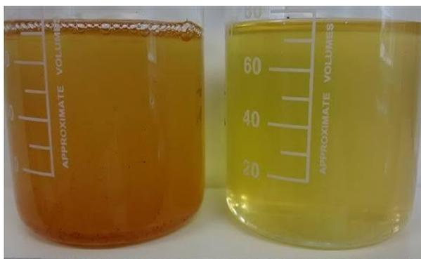
**Fig 23: The purification of bio-ethanol using activated Carbon.** The fig in the left is before purification and fig in the right is after purification.<sup>[6]</sup> The specific gravity of the ethanol changes from 0.85 to 0.81 ,which shows Removal of impurities from it.
