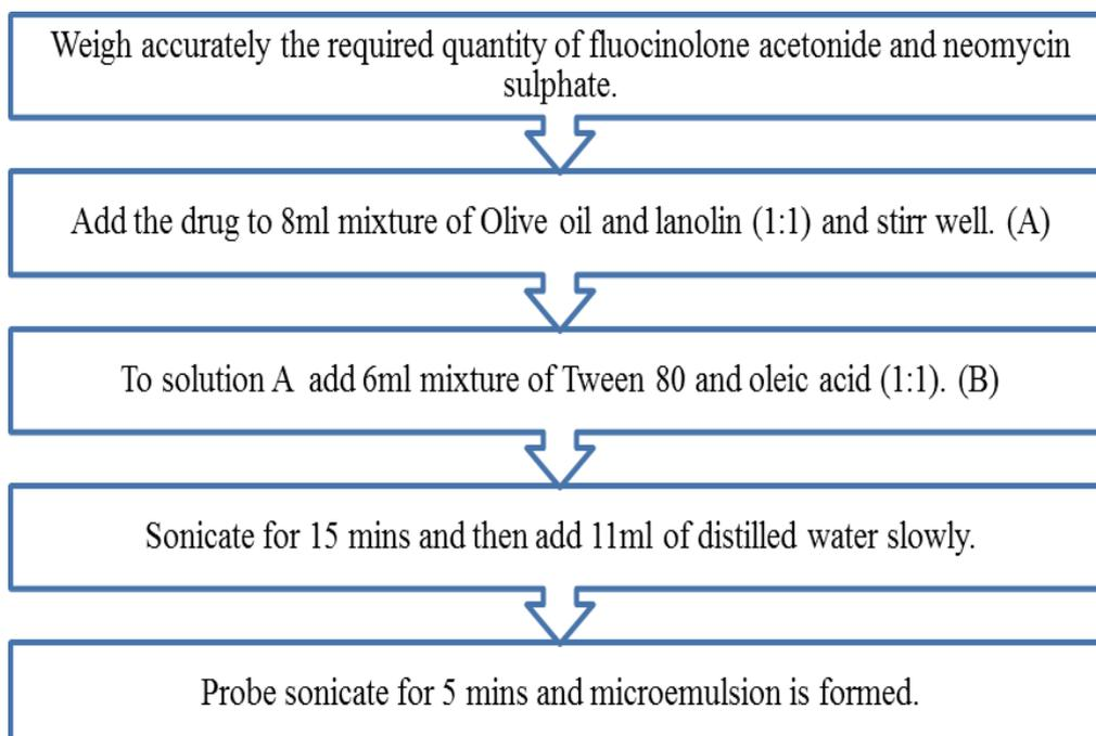
**Fig 3: Procedure for Preparation of Nana-Emulsion.**
