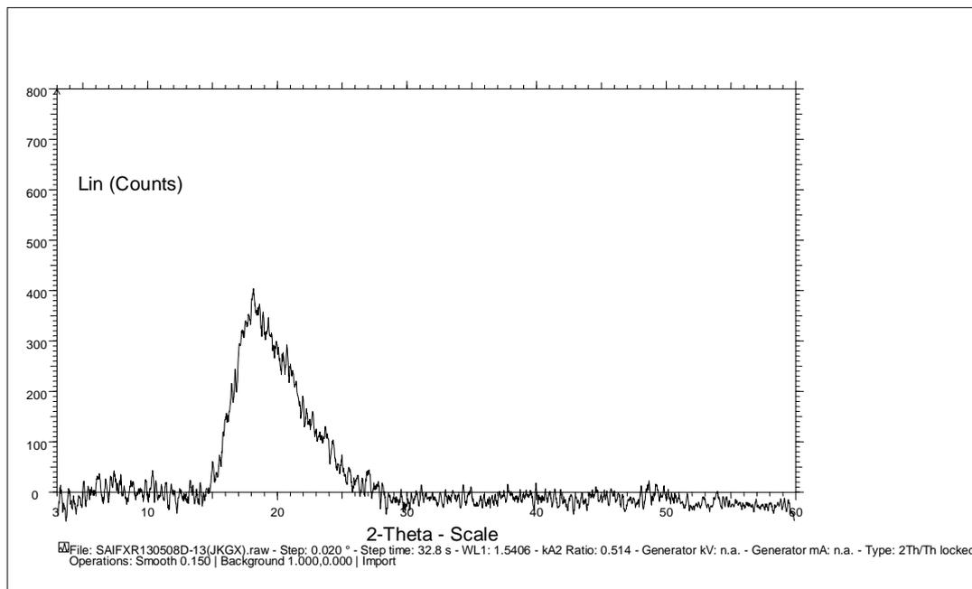
**Fig.7: X-Ray diffraction pattern of *Grevillea robusta* gum Scanning Electron Microscopy (SEM)**
