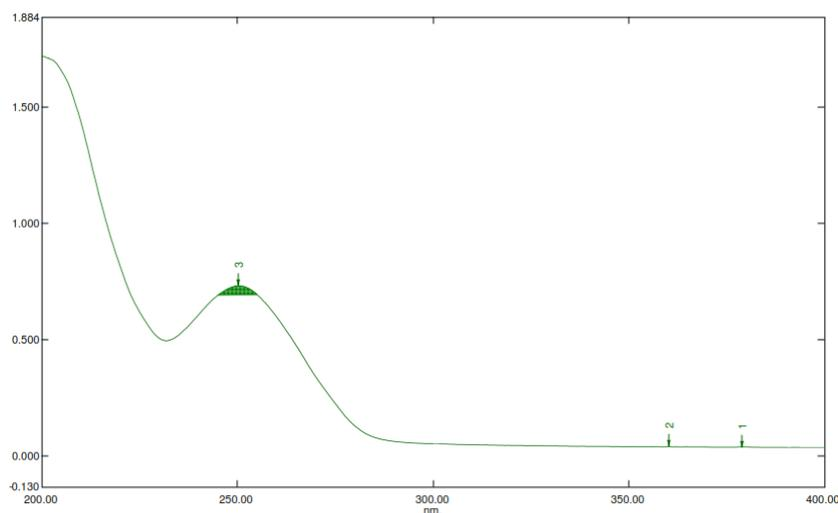
**Figure 7: Area under curve spectrum of Allopurinol**
