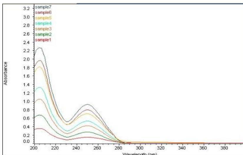
**Figure 3: Zero Order Spectrum (overlay) of Allopurinol.**
