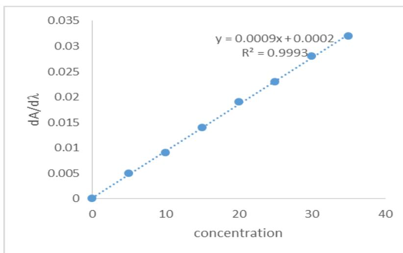
**Figure 6: Calibration curve of Allopurinol (first order).**
