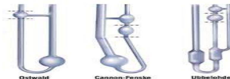
Fig. 4 Capillary viscometers Ostwald, Fenske, Ubbelohde
