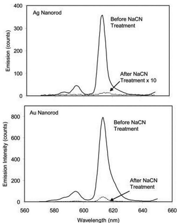
**Fig. 5** Emission spectral changes for the Eu(III) chelates on the Ag rods and gold rods in aqueous solution prior to and after NaCN treatment. The emission spectra were collected upon excitation at 380 nm. The gate pulse width was controlled to be 0.5 ms and the delay time was 0.1 ms.
