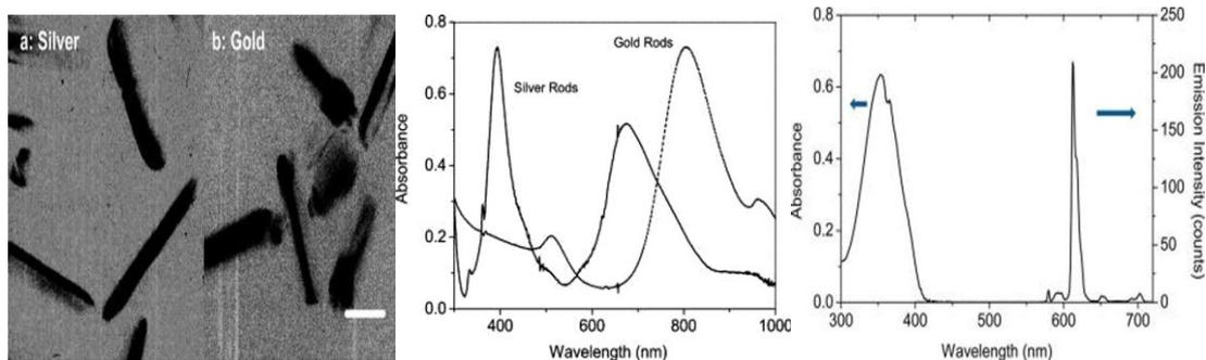
**Fig 1. Low-resolution TEM images of (a) silver and (b) gold nanorods. The scale bar in the image is 20 nm.**
