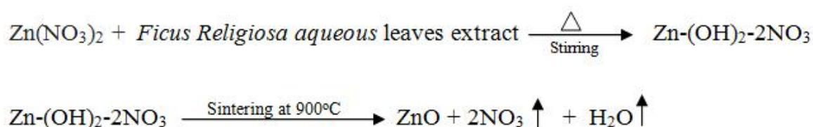
Zinc hydroxide nitrate is an intermediate product of the hydrolysis reaction, formed in the presence of H<sub>2</sub>O and OH<sup>-</sup> ions. It can be easily transformed into ZnO at higher temperature and with prolonged refluxing. Nitrate is water soluble and could therefore be removed from the end product. High purity ZnO nano-powder could therefore be obtained successfully by this green technique.<sup>[11]</sup>
