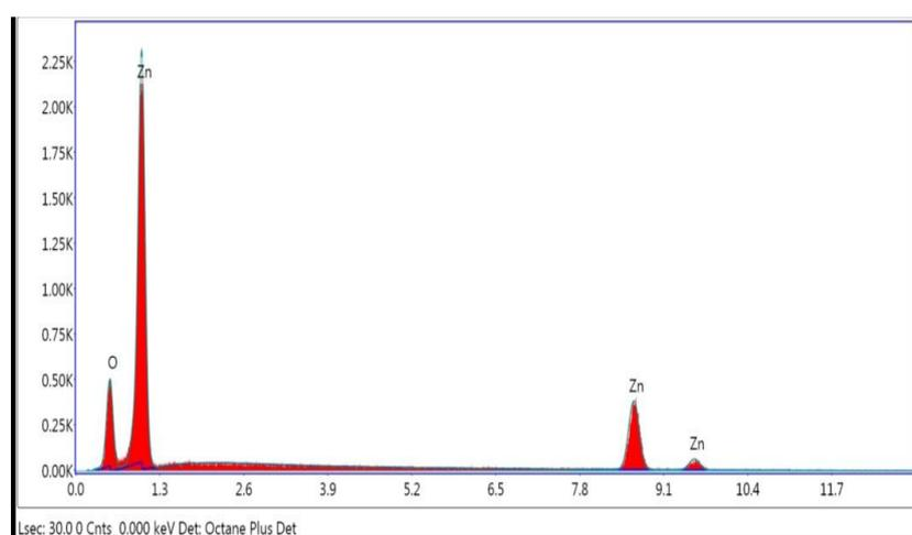
Figure 5: EDX graph of ZnO nanoparticles.
