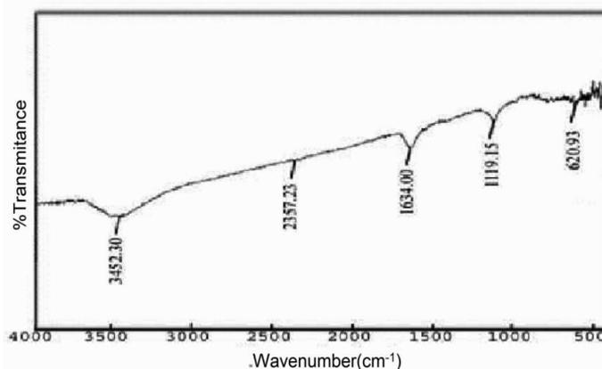
**Figure 2: FTIR spectra of ZnO nanoparticles.**
