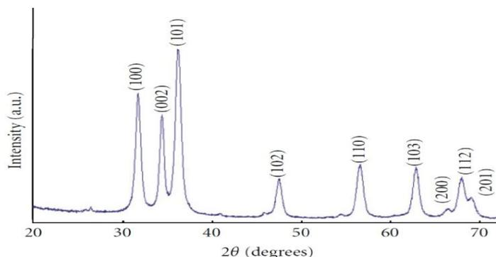
**Figure 3: XRD pattern of prepared ZnO nanoparticles.**
