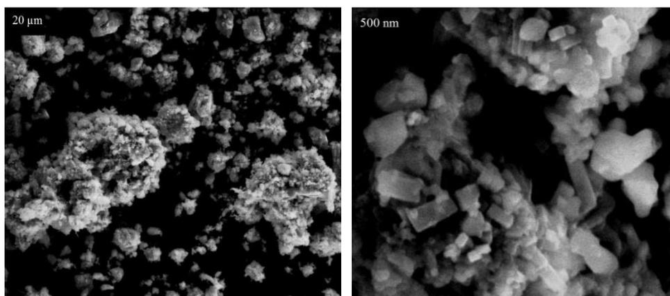
Figure 4: SEM pictures of ZnO nanoparticles at different magnifications.
