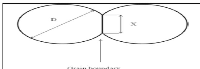
**Figure 1: Sketch of a model of the sintering of two particles.**
