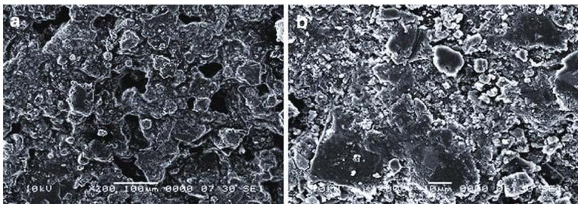
**Figure 3:** Scanning electron microscope images of a) unsintered and b) sintered tablet surfaces.
