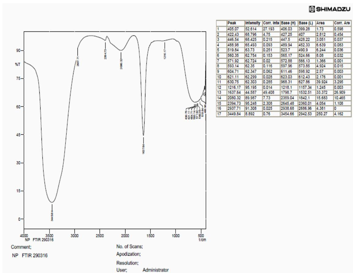
Fig 3: FTIR analysis of the synthesised Nanoparticle.
