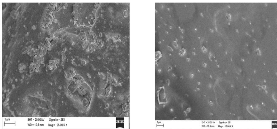
**Fig 4: SEM Micrograph of biosynthesized TiO<sub>2</sub> nanoparticles.**
