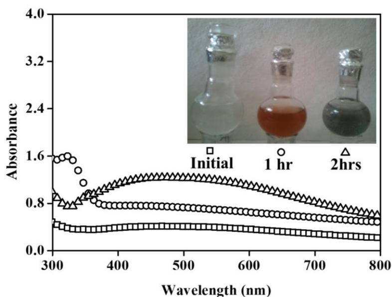
**Fig. 1.** UV-Visible absorption spectra of SNPs at different stages during synthesis of silver nanoparticles (SNPs) from *Ficus racemosa* latex (Inset photograph shows colour changes at each stage).
