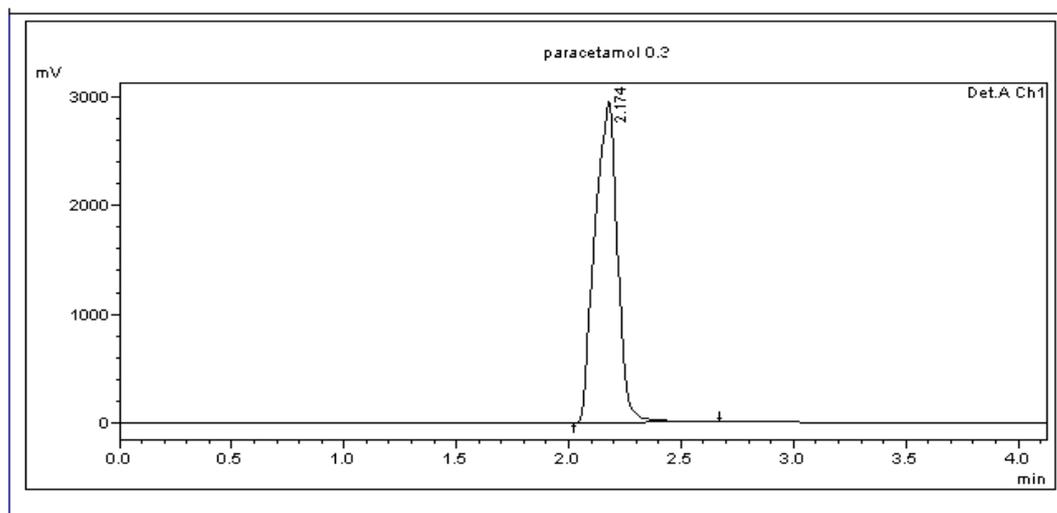
**Figure [2]: Typical chromatogram (paracetamol 50 µg/ml).**
