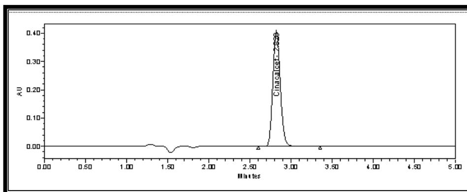
**Figure 03: Chromatogram of Cinacalcet in Tablet Solution.**
