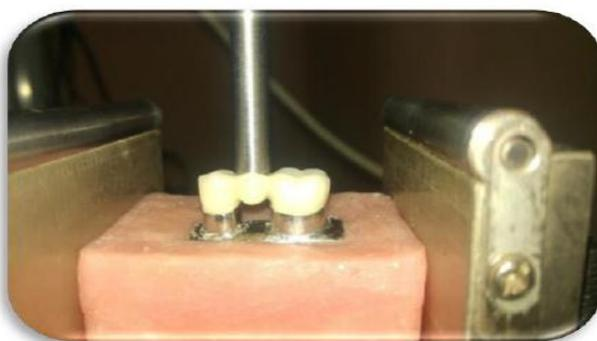
**Figure. (4): Bridge sample under load from steel ball of loading cell.**
