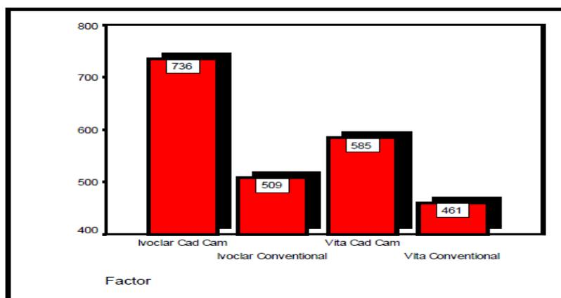
**Figure. (5): Plotting chart showing the mean values of fracture resistance of the four groups.**
