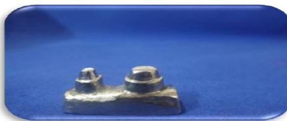
**Figure. (3): Master model from metal.**
