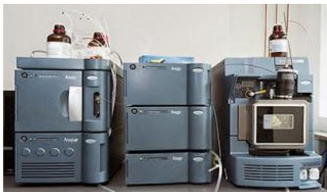
Figure 1: LC/MS/MS Instrument.<sup>[23]</sup>
