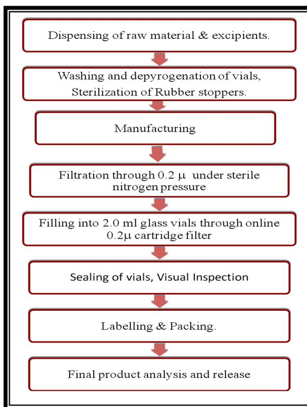
**Fig.:** Process flow diagram of parenteral dosage form
