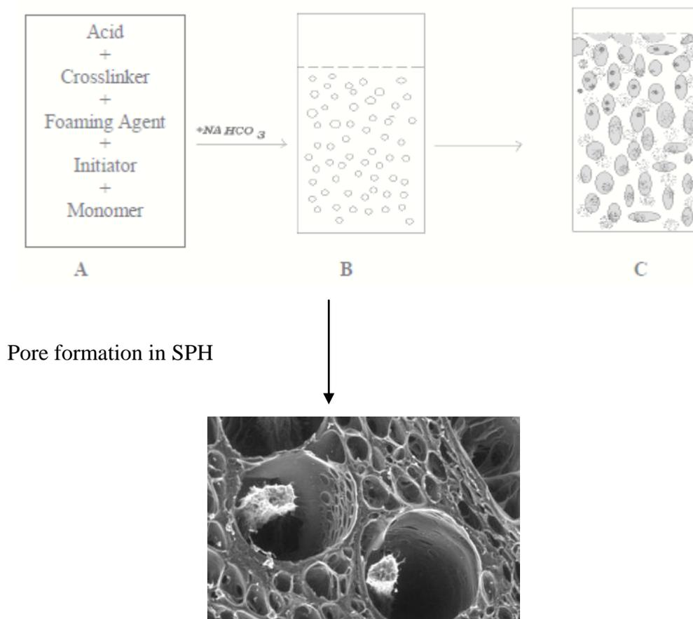
**Fig. 3 Schematic representation of the superporous hydrogel preparation.**
