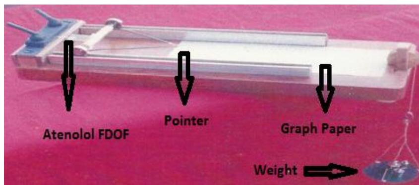
**Fig. 1.** Apparatus for the measurement of tensile strength and percentage elongation
