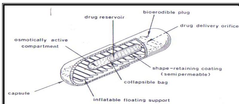
Figure no.9: The Osmotically controlled drug delivery device
