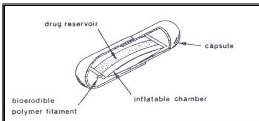
Figure no. 8: Inflatable Gastrointestinal Delivery Systems
