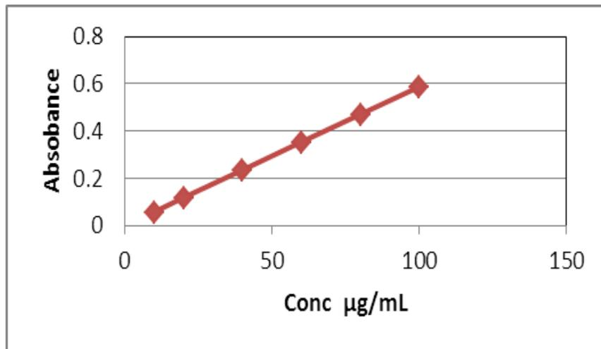
**Fig. 1: Standard curve of 5- fluorouracil**
