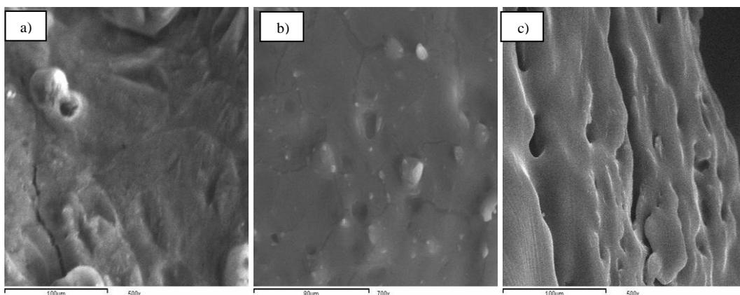
**Fig. 3. SEM of surface polymeric textures a) without 5-fluorouracil, b)after loading with 5-fluorouracil, and c) after releasing 5-fluorouracil in distilled water for 3days.**
