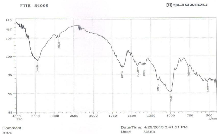
**Fig 2: FT – IR Spectrum of Sodium Starch Glycolate**
