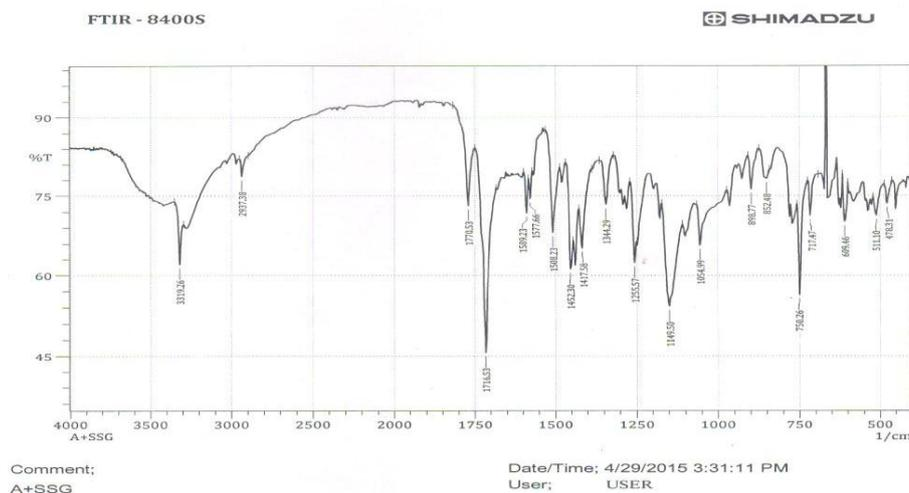
**Fig 3: FT – IR Spectrum of Aceclofenac + Sodium Starch Glycolate**
