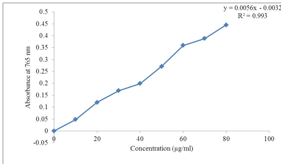
**Figure 1: Calibration curve of Gallic acid**
