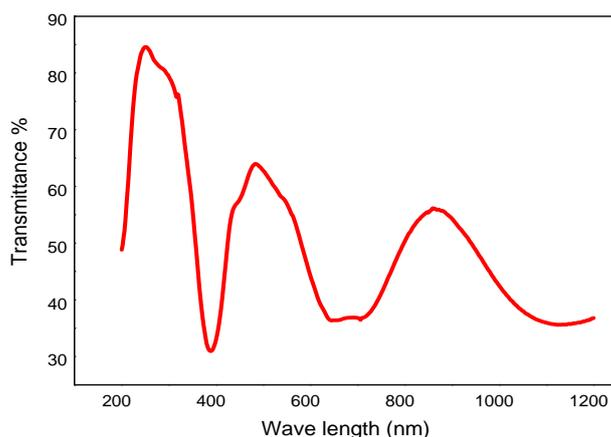
**Figure 3. UV Transmission graph of grown crystal**
