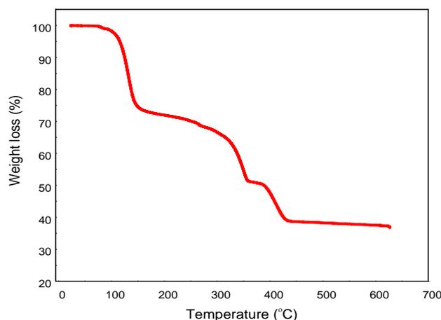
**Figure 4. TGA spectra of grown crystal**
