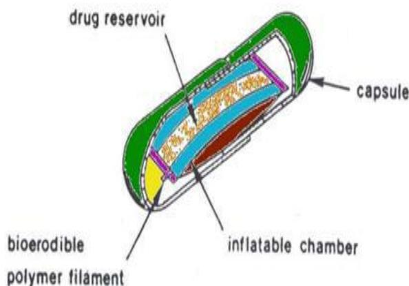
**Fig.9: Inflatable gastrointestinal delivery system**
