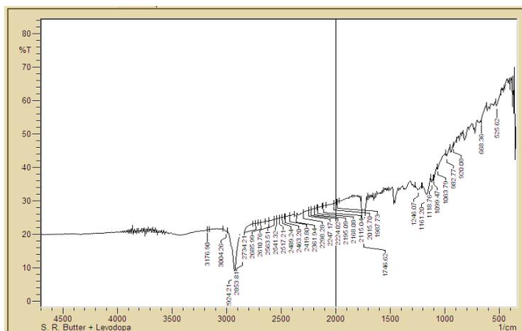
Fig. 5: IR spectrum of mixture of levodopa and S R butter
