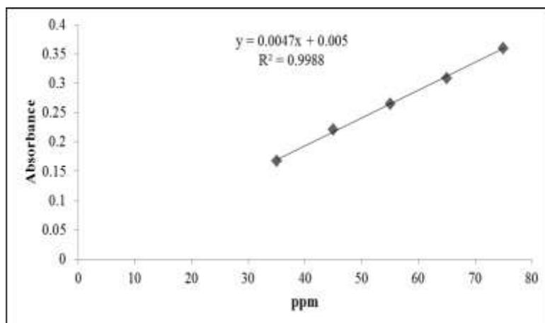
**Figure 3: Standard calibration curve of Atenolol Standard in 7.4 pH phosphate buffer**
