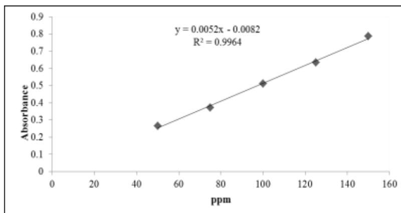
**Figure 2: Standard calibration curve of Atenolol Standard in 0.1N HCL**
